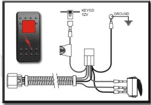
The Detroit Electrac is designed for vehicles with a 12-volt, negative ground electrical system. A wiring harness, ground wire and switch are provided with the Detroit Electrac.
