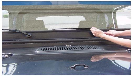
Step (17) Making sure your vehicle is still out of gear, turn the key to "accessory" and turn the wipers on. Make sure that everything is working properly. You may need to adjust the position again so they lay flat after operating it for a few seconds.
