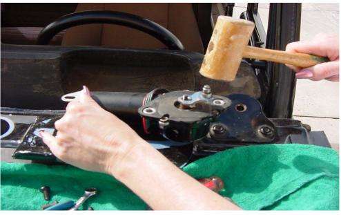
**Step (10)** Install the new motor arm (WB-EMBSC-A), oriented to the same angle as the original, using the pen mark you made in Step 8 for reference.
