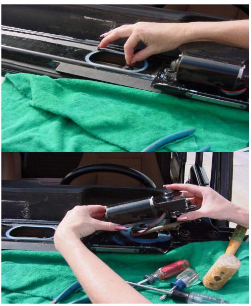
Step (12) Attach the motor-side linkage to the windshield-side linkage, remembering to put the other clip back on. Now would be a good time to put a few drops of oil on the remaining linkage joints.
