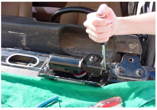
**Step (5)** Drape a towel or blanket over you window so you don't scratch the window. Slide the wiper motor out, and the linkage will slide out with it.
