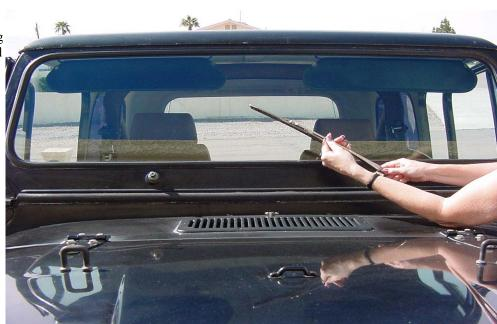
Step (2) Fold the window down to get access to the wiper motor. Note: it takes a bit more time if you have a hardtop installed. Remove the bolts, only loosening the back bolts that hold the hardtop on. Have someone help you lift the front of the top a little so it clears the lip of the window frame. Now you can fold the window down.
