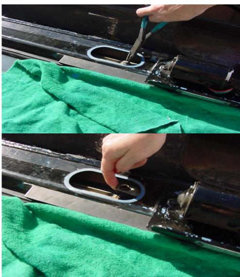
**Step (4)** Remove the 3 Torx screws from the wiper motor (you don't have to disconnect the wires). You just need to be able to slide the motor and linkage out. There may be a small screw that holds the wire to the bottom of the frame, in which case you might have to remove the screw to give you the slack to pull the motor out.
